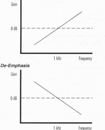
The emphasis curve is steep—it amplifies or attenuates at 6db/octave. Notice that at 1 kHz, the level is the same regardless of whether or not the signal has been pre-emphasized or de-emphasized. This is the reference level used to make all measurements. Because of the steep emphasis function, all transmit and receive level adjustments must be made using the 1kHz reference!
