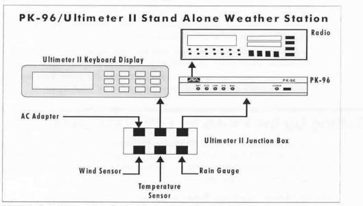
FIGURE 3: Illustrates components of a stand alone packet weather station
