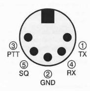
**PK-96 to Radio Cable Connections**
