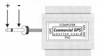
Notice the words on the outside of the rectangle; they say TNC, Computer, and GPS. This is how the Cable should be connected.
